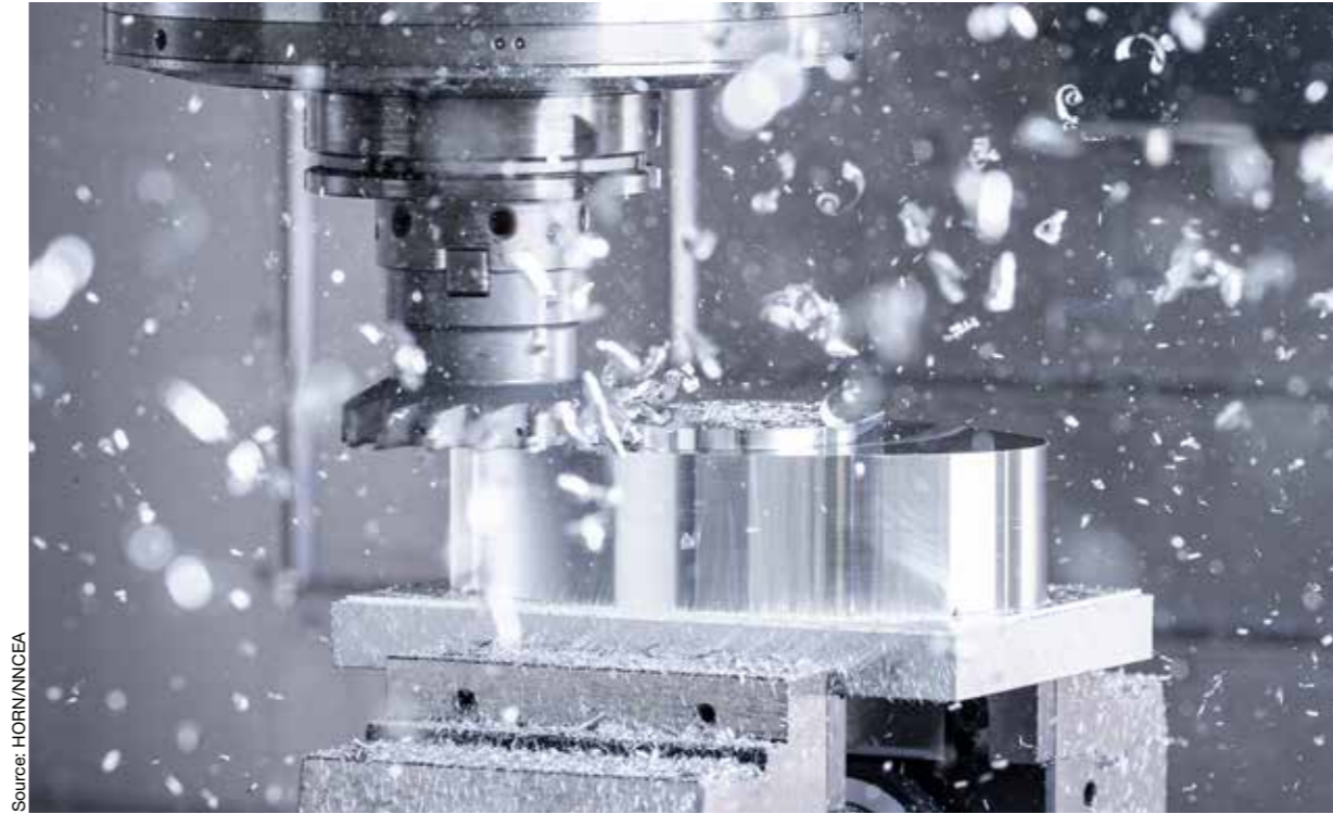
The Horn high-performance PCD grade consists of a sophisticated mixture of diamond grains of different sizes.
